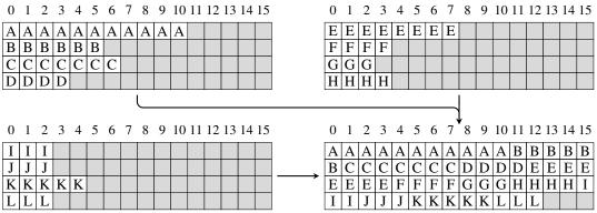
Figure 3: Efficient sample packing using flash\_attn\_varlen\_func
